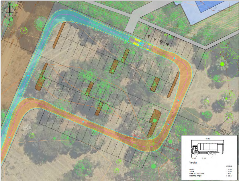
Figure 18 Swept Path Analysis – Waste Truck Internal Circulation
